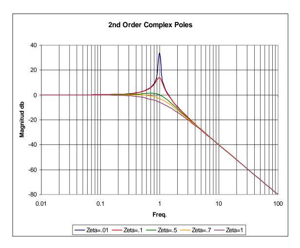
We still get the -40 db/decade roll-off, but the response of the system about the break frequency varies significantly as a function of zeta. When zeta=.01, there exists an extremely narrow selectivity bandwidth about the break frequency. When zeta=.01 the time constant, in this case, equals 100s and the system impulse response dies out at 600s. When  $\zeta = 1$ , the system is just a 2nd order repeated real pole filter at a break frequency of 1.
