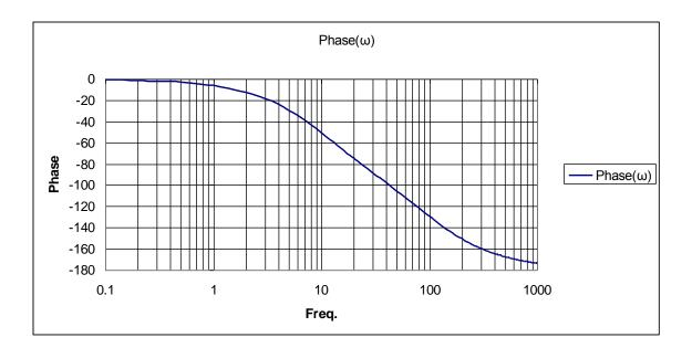
Again, another pattern that is emerging is that each pole contributes a -90° phase shift at the output. n poles =  $n^*(-90^\circ)$  shifts. That fact allows you to predict the terminal phase shift as  $\omega \rightarrow \infty$ .
