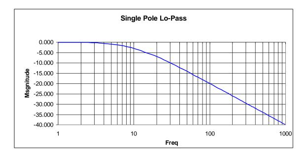
As can be seen from the above  $Bode^3$  (Bo-dee) plot the output magnitude begins to roll off as  $\omega$  approaches the break frequency (in this case 10 rads/s). At the break frequency, the magnitude is at -3db and rolls off at -20db per decade. Please note that this technique plots the output magnitude versus frequency, but does not address the frequency content of the output. That aspect of system response is left to Fourier analysis which is the subject of a different set of modules.
