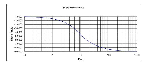
As expected for this circuit, the phase of the output with respect to the input varies from 0 to -90° as a function of  $\omega(\arctan \infty is 90°)$ . At very low frequencies the capacitor acts like an open and the input is the output. At high frequencies the capacitor begins to act like a short, and by the voltage division rule an ever larger percentage of the input is dropped across the resistor, while the phase of the voltage that is dropped across the capacitor approaches the -90° rail.
