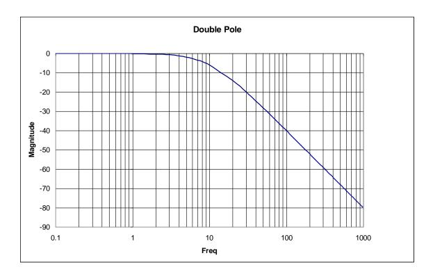
Also notice that at the break frequency the magnitude is down by -6db, i.e., - 3dbfor each pole.
