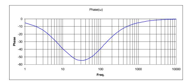
It was simple to predict that the terminal phase change would sum to zero as  $\omega \rightarrow \infty$ , since  $-90^{\circ}+90^{\circ}=0$ . Since the two break frequencies are 10 rads/s and 100 rads/s we should expect maximum phase changes  $\left(\frac{d\phi}{d\omega}\right)$  to occur within that range of frequencies; from the plot it is seen that there is indeed a minimum accompanied by a sign change.
