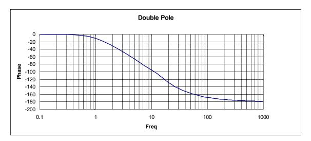
Again the phase begins a zero, but ends at -180, or double the single pole, and is verified by the phase equation above. That will hold throughout, n poles equals output phase tending towards  $n^{*}(-90)$ . Conversely, n zeros will drive the output phase towards  $n^{*}(+90)$ .
