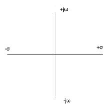
For the present, we will leave this topic, but we will return to it in later modules and use this coordinate system in pursuit of stability in circuit design. For reasons of stability, we will restrict the signs in the quadratic to be positive, i.e. the real parts of the roots lie to the left of the  $j\omega$  axis. That is a general, and prudent, design constraint. A little thought about the behavior of f(t) as a function of  $e^{+\alpha}$  provides the reason.
