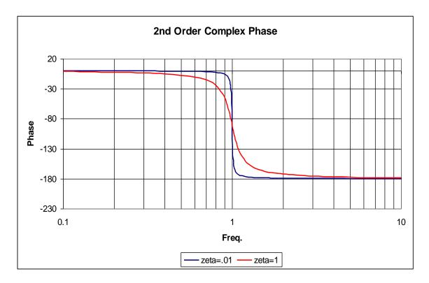
When the resonant frequency is changed, all that changes in the pattern is the frequency that the peaks occur at in the magnitude plot, and the frequency that holds the  $-90^{\circ}$  spot in the phase plot.
