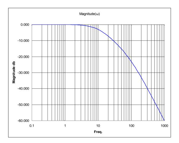
As expected the roll-off between 10 and 100 rads/s s is -20db per decade, whereas the roll-off between 100 and 1000 rads/s is -40db per decade. The pattern that is emerging is that each pole contributes a -20db per decade roll-off beginning at the break frequency. If a -100db per decade roll-off is needed, then you will need a 5 pole filter. -ndb per decade requires n/20 poles.
