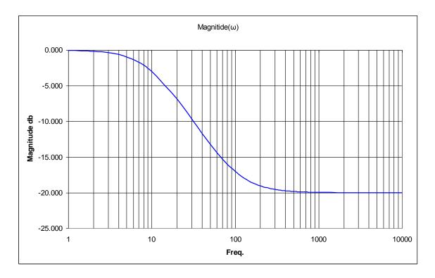
From the expression that the magnitude versus frequency plot is constructed, we should expect a -20db roll-off beginning at 10 rads/s and a +20db roll-on at 100 rads/s.
