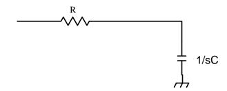
In the above circuit (a single pole lo-pass) assume  $V_{out}$  is taken across the capacitor and that RC=.1, in that case then:
